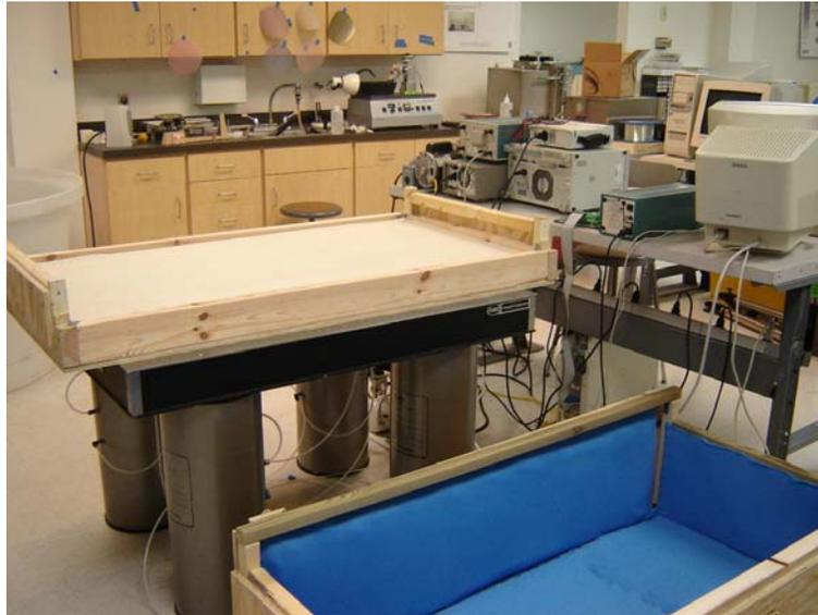
Fig. A.4: Sandbox and Acoustic Enclosure
