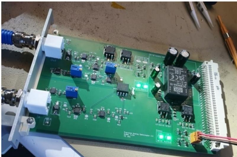
The circuit and the board is a replica of a project by Todd Meyrath which can be found [here](#). The central optocoupler circuit was inspired by fig. 17 of the [datasheet of the HCNR200](#).
