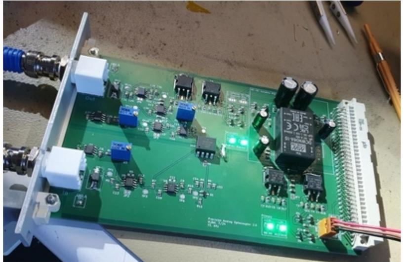
The circuit and the board is a replica of a project by Todd Meyrath which can be found [here](#). The central optocoupler circuit was inspired by fig. 17 of the [datasheet of the HCNR200](#).
